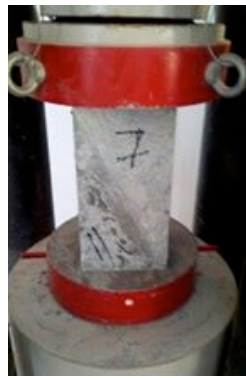
Figure 3: Slant shear test set-up.
