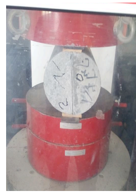
Figure 4: Splitting tensile test set-up.
