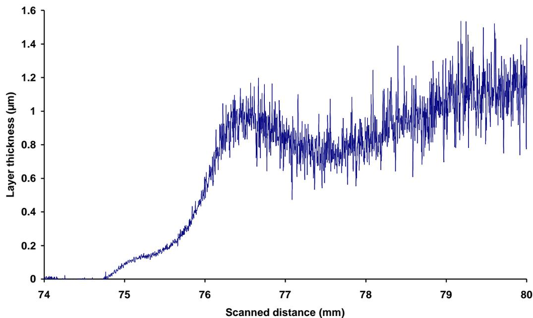
Figure 5: Tallysurf thickness profile of an electrodeposited CuInTe<sub>2</sub> layer.
