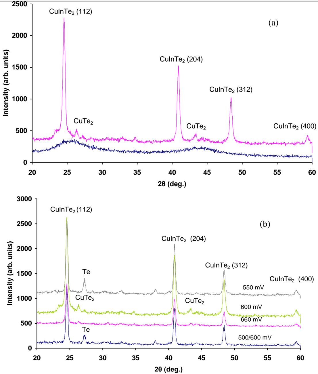
Figure 3: XRD pattern of (a) As-deposited and heat treated CuInTe<sub>2</sub> layers, and (b) heat treated CuInTe<sub>2</sub> layers electrodeposited at different cathode voltages.
