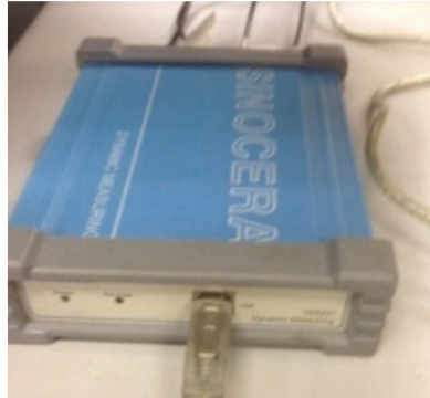
Figure 8 Data acquisition equipment (model YE6261B)
