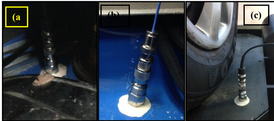
Figure 9 (a) Sensor position on front wheels (b) sensor position on rear wheels and (c) sensor position on the shaker base.
