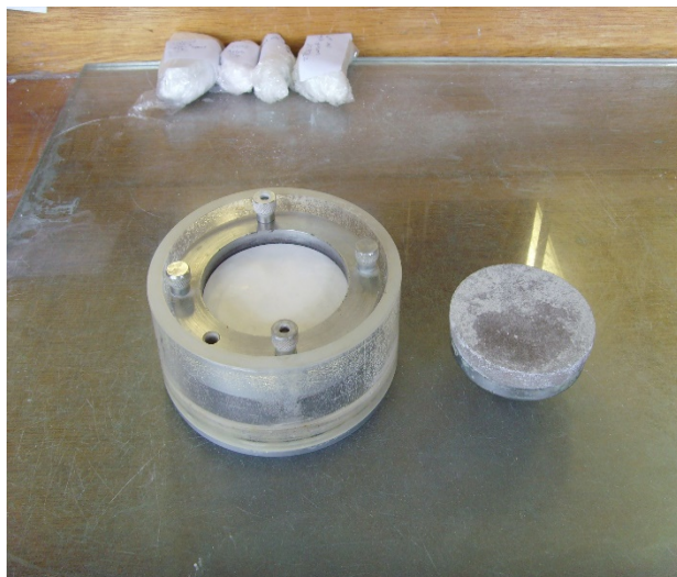
Figure 3. Soil sample placement within Oedometer cell
