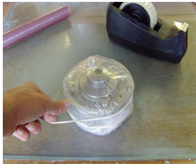
Figure 4. Isolation of sample from surrounding humidity
