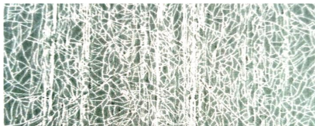
Figure 3.4 A: Scanning Electron Micrograph at 20 kV of the coating produced in solution IV
