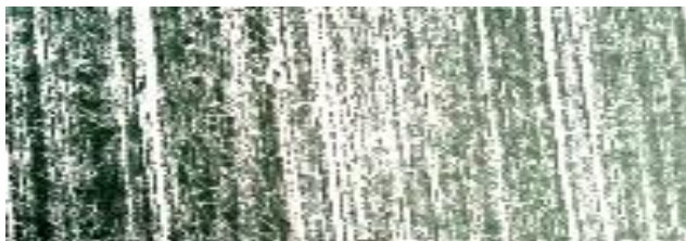
Figure 3.5.2A: Scanning Electron Micrograph at 20 kV of the coating produced in solution V
