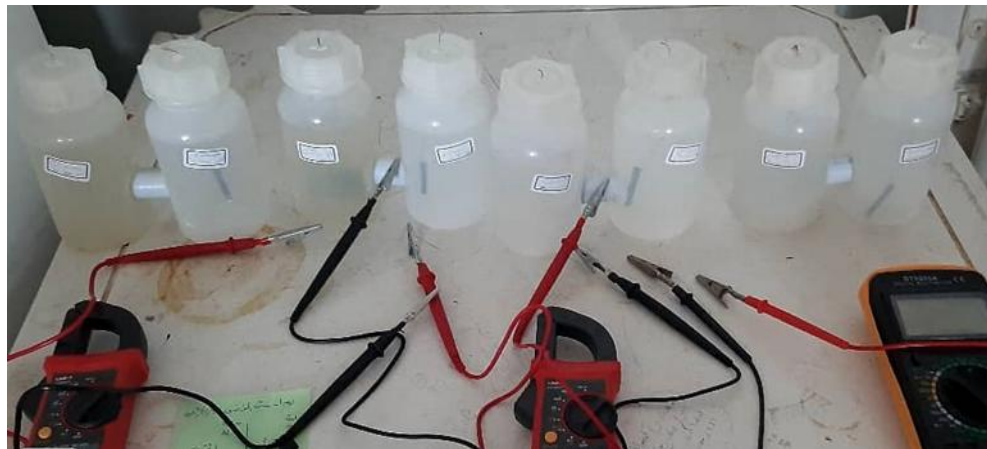
Figure 3 Double chambered waste water microbial fuel cells MFCs
